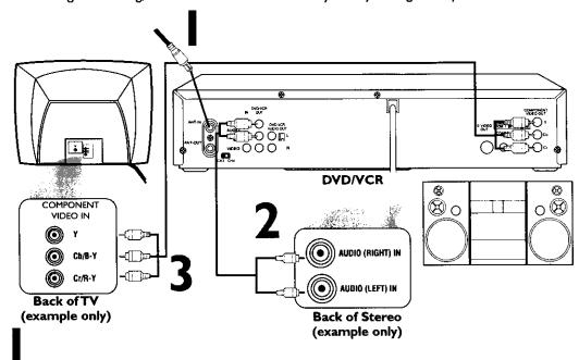
Connect the antenna or cable to the ANT-IN (Antenna In) jack of your DVD/VCR.
